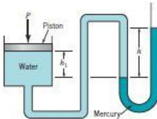
7. The pressure of water flowing through a pipe is measure by the arrangement shown below. For the values given, calculate the pressure in the pipe.
